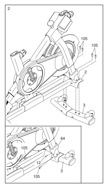
3. Attach the Rear Stabilizer (4) to the Base (2) with four M10 x 20mm Screws (105); **do not fully tighten the Screws yet.**
