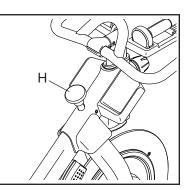
To change the resistance of the pedals, press the buttons on the right handlebar (see step 3 on page 22). To stop the flywheel, press the brake knob (H) downward. The flywheel will quickly come to a complete stop.
