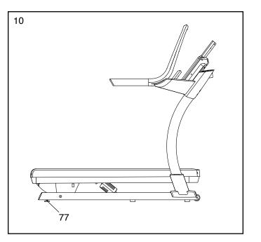
11. Make sure that all parts are properly tightened before you use the incline trainer. Keep the included tools in a secure place. One of the hex keys is used to adjust the walking belt (see pages 28–29). To protect the floor or carpet from damage, place a mat under the incline trainer. To avoid damage to the console, keep the incline trainer out of direct sunlight.
