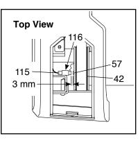
**gap between the Magnet and the Reed Switch must be about 3 mm (1/8 in.).** If necessary, loosen the #8 x 3/4" Clip Screw (116), move the Reed Switch slightly, and then retighten the Clip Screw. Then, see the larger drawing above and reattach the Left Foot Rail Cover (44) with the #8 x 3/4" Screw (5). Then, run the incline trainer for a few minutes to check for a correct speed reading.
