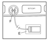
for the console to be ready for use. IMPORTANT: In an emergency, the key can be pulled from the console, causing the walking belt to slow to a stop. Test the clip by carefully taking a few steps backward; if the key is not pulled from the console, adjust the position of the clip.
