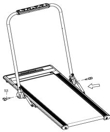
Step 3: Take the side handrail, and insert the axle into hole.
