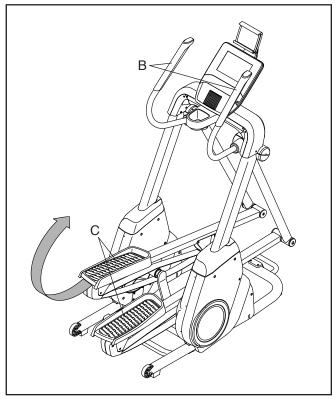
To dismount the elliptical, wait until the pedals (C) come to a complete stop. Note: The elliptical does not have a freewheel; the pedals will continue to move until the flywheel stops. When the pedals are stationary, step off the higher pedal first. Then, step off the lower pedal.
