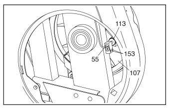
Then, slightly loosen the two M4 x 25mm Screws (153) and slide the Reed Switch (55) slightly closer to or away from the Magnet (113).
