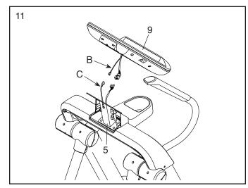
12. **Tip: Avoid pinching the wires.** Attach the Console (9) to the Console Bracket (5) with four M4 x 16mm Screws (143); **start all the Screws, and then tighten them.**
